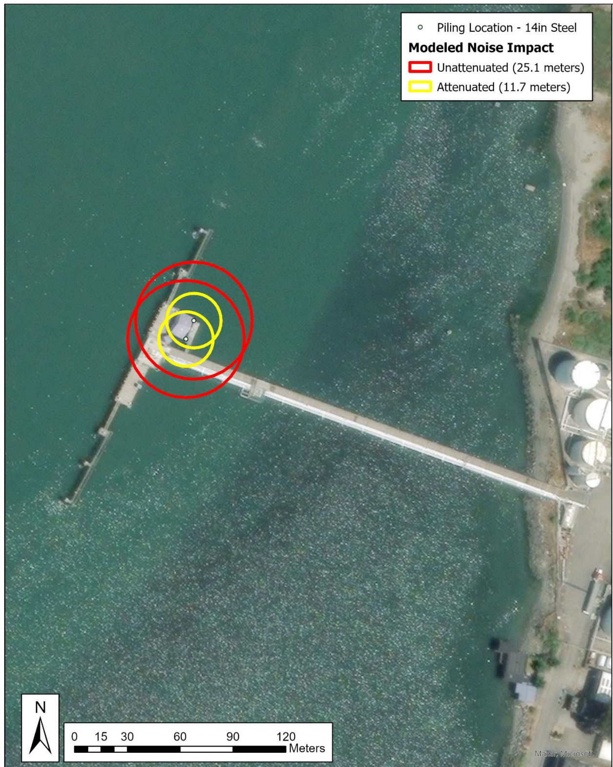
Figure 7. Injury Zones for Fish Weighing < 2g, 14-Inch Pilings
